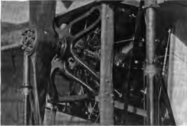
THE 14-CYL. 100-H. P. GNOME MOTOR OF CLAUDE GRAHAME-WHITE'S BLERIOT RACER WITH WHICH HE WON THE GORDON-BENNETT CUP RACE ON OCT. 29TH, 1910, AT BELMONT PARK
